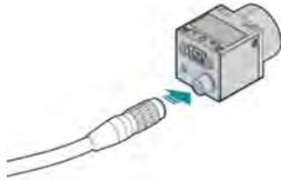
GPIO can be used for power, trigger, pulse width modulation, serial input output, and strobe.
