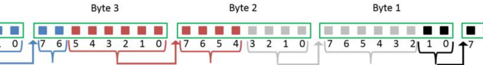
Figure 1. Packing two 10-bit pixels into three bytes.
