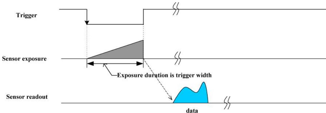
Figure 7.2: Trigger Mode 1 (“Bulb Shutter Mode”)
