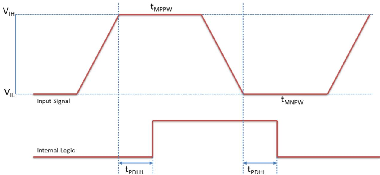
Table 6.8: Opto-isolated Input Performance ( $V_{CC}$  = varying pk-pk)
