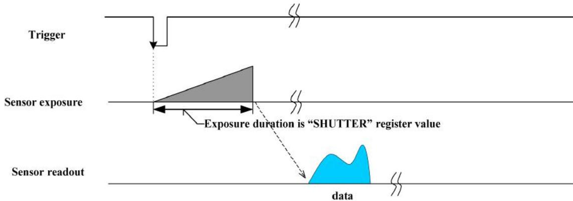
Figure 7.1: Trigger Mode 0 (“Standard External Trigger Mode”)
