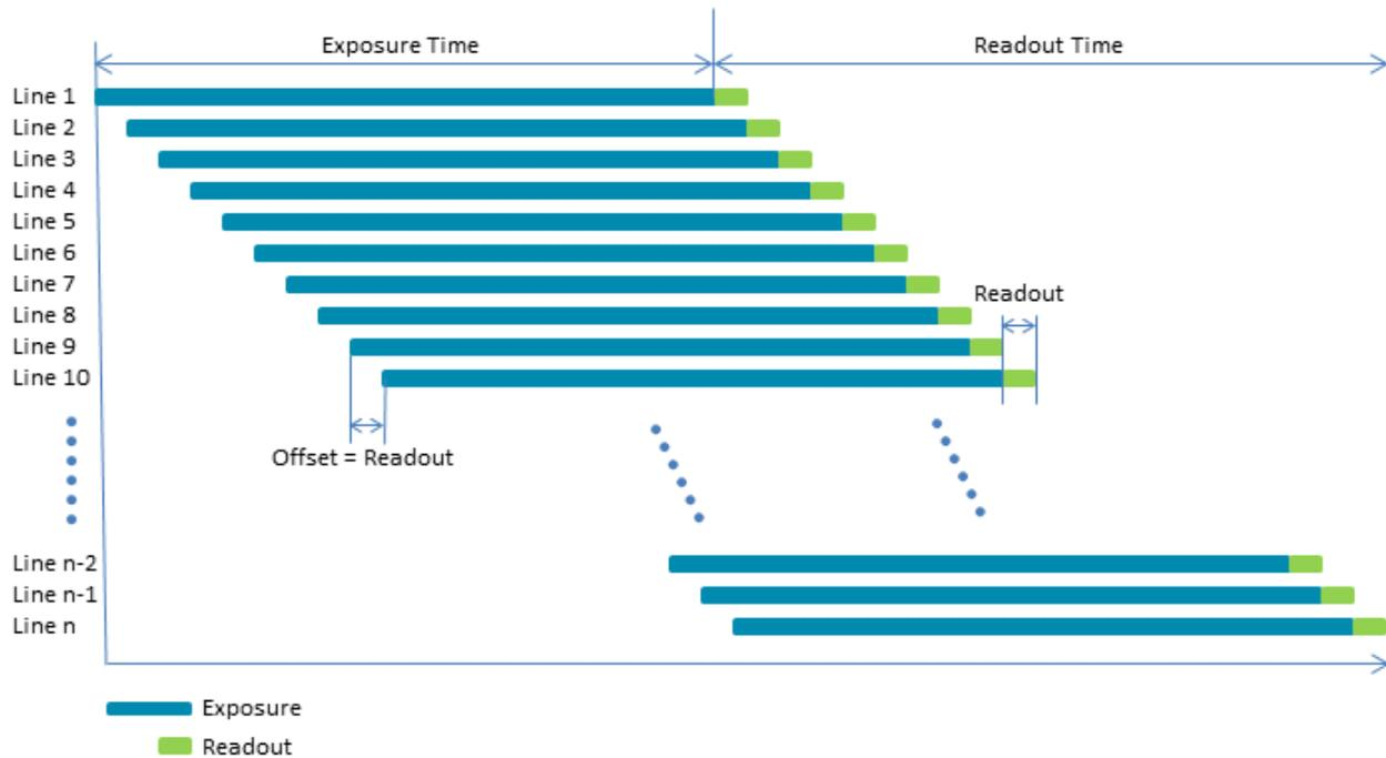
One advantage of a rolling shutter is increased sensitivity. However, because exposure starts at different times throughout the frame, there are known artifacts such as skew, wobble, and partial exposure. For more information, see [Rolling Shutter Artifacts](#).
