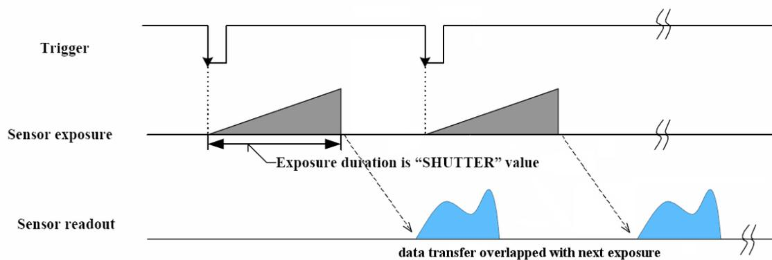
Figure 7.4: Trigger Mode 14 (“Overlapped Exposure/Readout Mode”)
