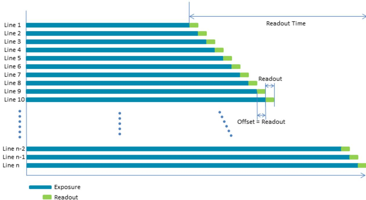
An advantage of a rolling shutter with global reset is a reduction in image artifacts typical of rolling shutters such as skew and wobble. However, because exposure lengthens throughout the frame, there may be a gradual increase in brightness from top to bottom of an image. This gradient can be diminished or even eliminated by using a strobe flash. For more information, see [Rolling Shutter Artifacts](#).
